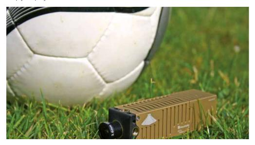
The INCA intelligent camera is small, robust and delivers HD quality images together with additional data, like acceleration, temperature and pulse. © Fraunhofer IIS | Picture in color and printing quality: www.iis.fraunhofer.de/pr/.
